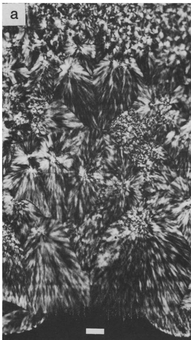
Figure 1 (a) B-315-M, section taken immediately next to stub prepared for etching, seen in circularly polarized light. (b) Same specimen, stub etched with 2% w/v potassium permanganate in orthophosphoric acid ex-bottle, showing accurate presentation of spherulitic detail corresponding to the section in Figure 1a , but with irregular pitting of the surface. Scale bars = 10 μm
